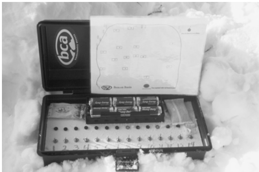
Beacon Basin control panel.
